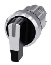
Selector switch, illuminable, 22 mm, round, metal, shiny, white, selector switch, long, 3 switch positions I>O<II, momentary contact on the left, latching on the right, actuating angle 2x45°, 10:30h/12h/13:30h, Z=50-unit packaging
