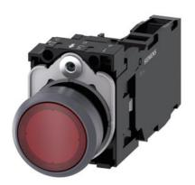
Illuminated pushbutton, 22 mm, round, plastic with metal front ring, red, pushbutton, flat, momentary contact type, with holder, 1 NO+1 NC, LED module with integrated LED 110 V AC, screw terminal, with laser labeling, inscription or symbol Customer-specific selection with SIRIUS ACT configurator (CIN)
