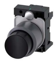
Pushbutton, compact, with extended stroke (12 mm), 22 mm, round, plastic with metal front ring, black, pushbutton, high, momentary contact type, with holder, with laser labeling, upper case and lower case, always upper case at beginning of line
