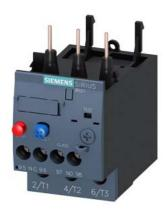
Overload relay 5.5...8.0 A Thermal For motor protection Size S0, Class 10 Contactor mounting Main circuit: Screw Auxiliary circuit: Screw Manual-Automatic-Reset
