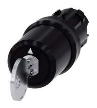
Key-operated switch BKS, 22 mm, round, plastic, lock number S1, with 2 keys, 3 switch positions I-O-II, latching, actuating angle 2x45°, 10:30h/12h/13:30h, Key removal I+O+II, with laser labeling, upper case
