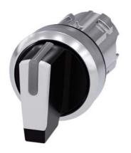
Selector switch, illuminable, 22 mm, round, metal, shiny, white, selector switch, short, 3 switch positions I-O<II, left latching, right momentary contact type, actuating angle 2x45°, 10:30h/12h/13:30h, Z=50-unit packaging
