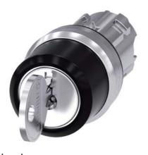
RONIS key-operated switch, 22 mm, round, metal, shiny, lock number SB30, with 2 keys, 3 switch positions I-O<II, left latching, right momentary contact type, actuating angle 2x45°, 10:30h/12h/13:30h, key removal O+I, possible special locks: SB31, 421, 455, with laser labeling, upper case and lower case, always upper case at the beginning of the word
