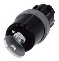
key-operated switch Siemens, 22 mm, round, plastic with metal front ring, lock number SSG10, with 2 keys, 2 switch positions O<I, momentary contact type, actuating angle 45°, 10:30h/12h, key removal O, with laser labeling, inscription or symbol customer-specific selection with SIRIUS ACT configurator (CIN)
