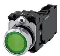
Illuminated pushbutton, 22 mm, round, metal, shiny, green, pushbutton, flat, momentary contact type, with holder, 1 NO+1 NC, LED module with integrated LED 110 V AC, screw terminal, with laser labeling, lower case
