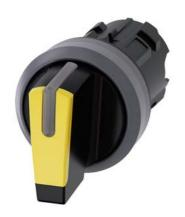
Selector switch, illuminable, 22 mm, round, plastic with metal front ring, yellow, selector switch, short, 3 switch positions I-O-II, latching, actuating angle  $2x45^{\circ}$ , 10:30h/12h/13:30h, Z=50-unit packaging
