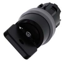
Key-operated switch O.M.R, 22 mm, round, plastic with metal front ring, lock number 73034, black, with 2 keys, 2 switch positions O<I, momentary contact type, Actuating angle 45°, 10:30h/12h, key removal O, with laser labeling, inscription or symbol Customer-specific selection with SIRIUS ACT configurator (CIN)
