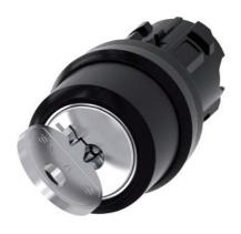
RONIS key-operated switch, 22 mm, round, plastic, Lock No. 421, with 2 keys, 2 switch positions O-I, latching, actuating angle 90°, 10:30h/13:30h, key removal O+I, with laser labeling, inscription or symbol Customerspecific selection with SIRIUS ACT configurator (CIN)
