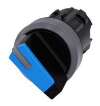
Selector switch, illuminable, 22 mm, round, plastic with metal front ring, blue, selector switch, short, 2 switch positions O-I, latching, actuating angle 90°, 10:30h/13:30h, with laser labeling, upper case and lower case, always upper case at beginning of line
