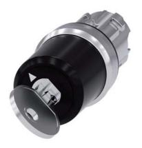
key-operated switch Siemens, 22 mm, round, metal, shiny, lock number SSG10, with 2 keys, 2 switch positions O-I, latching, actuating angle 90°, 10:30h/13:30h, key removal O+I, with laser labeling, inscription or symbol customer-specific selection with SIRIUS ACT configurator (CIN)
