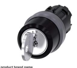
RONIS key-operated switch, 22 mm, round, plastic with metal front ring, lock number 455, with 2 keys, 3 switch positions I-O-II, latching, actuating angle 2x45°, 10:30h/12h/13:30h, Key removal I+O+II, with laser labeling, lower case
