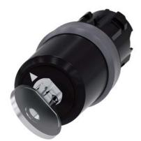
Key-operated switch BKS, 22 mm, round, plastic with metal front ring, special lock, with 2 keys, 2 switch positions O-I, latching, actuating angle 90°, 10:30h/13:30h, key removal I, Note: BKS locking systems E1 - E25 supplied without key
