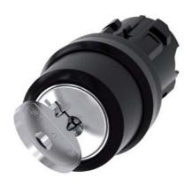
RONIS key-operated switch, 22 mm, round, plastic, Lock No. 421, with 2 keys, 2 switch positions O-I, latching, actuating angle  $90^\circ$ , 10:30h/13:30h, key removal O+I, with laser labeling, lower case
