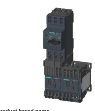
Load feeder fuseless, Reversing duty 400 V AC, Size S00 1.80...2.50 A 24 V DC Spring-type terminal for installation on standard mounting rail (also fulfills type of coordination 1) Type of coordination 2, Iq = 150 kA 1 NC (contactor)
