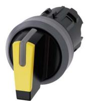
Selector switch, illuminable, 22 mm, round, plastic with metal front ring, yellow, selector switch, short, 3 switch positions I-O-II, latching, actuating angle 2x45°, 10:30h/12h/13:30h, with laser labeling, upper case and lower case, always upper case at the beginning of the word
