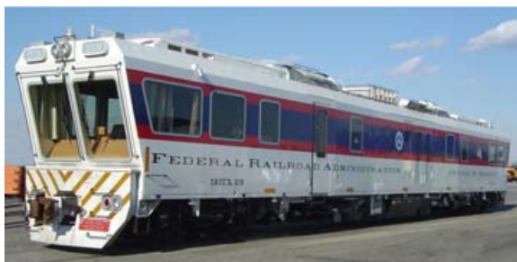
Track Inspection Car
