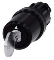
keyswitch BKS, 22 mm, round, plastic, special lock, with 2 keys, 3 switch positions I-O-II, latching, actuating angle  $2x45^{\circ}$ , 10:30h/12h/13:30h, key removal I+O+II, note: for the BKS locking systems E1 - E25 supplied without key
