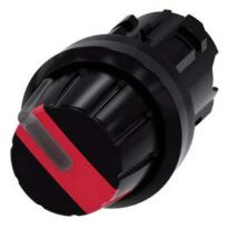
Selector switch, illuminable, 22 mm, round, plastic, red, Rotary knob, 2 switch positions O-I, latching, actuating angle 90°, 10:30h/13:30h, with laser labeling, upper case and lower case, always upper case at the beginning of the word
