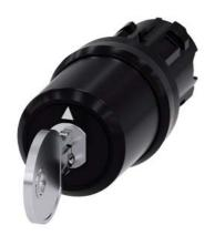
Key-operated switch BKS, 22 mm, round, plastic, lock number S1, with 2 keys, 3 switch positions I-O<II, left latching, right momentary contact type, actuating angle 2x45°, 10:30h/12h/13:30h, key removal I, with laser labeling, upper case
