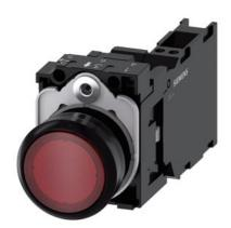
Illuminated pushbutton, 22 mm, round, plastic, red, pushbutton, flat, momentary contact type, with holder, 1 NO+1 NC, LED module with integrated LED 110 V AC, spring-type terminal, with laser labeling, upper case and lower case, always upper case at beginning of line
