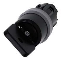
Key-operated switch O.M.R, 22 mm, round, plastic with metal front ring, lock number 73034, black, with 2 keys, 2 switch positions O<I, momentary contact type, Actuating angle 45°, 10:30h/12h, key removal O, with laser labeling, upper case
