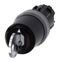
Key-operated switch IKON, 22 mm, round, plastic with metal front ring, lock number 360012K1, with 2 keys, 3 switch positions I-O-II, latching, actuating angle  $2x45^{\circ}$ , 10:30h/12h/13:30h, key removal O, with laser labeling, upper case and lower case, always upper case at the beginning of the word
