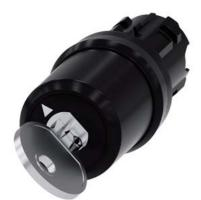
key-operated switch Siemens, 22 mm, round, plastic, lock number SSG10, with 2 keys, 2 switch positions O-I, latching, actuating angle 90°, 10:30h/13:30h, key removal O, with laser labeling, upper case and lower case, always upper case at beginning of line
