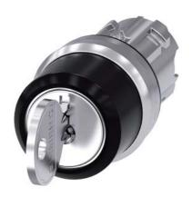
RONIS key-operated switch, 22 mm, round, metal, shiny, special lock, with 2 keys, 3 switch positions I-O-II, latching, actuating angle 2x45°, 10:30h/12h/13:30h, Key removal I+O+II, possible special locks: SB31, 421, 455
