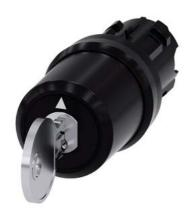
Key-operated switch BKS, 22 mm, round, plastic, Lock No. E9 (VW), without key, 3 switch positions I-O-II, latching, actuating angle 2x45°, 10:30h/12h/13:30h, Key removal I+O+II, with laser labeling, lower case
