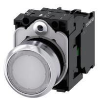
Illuminated pushbutton, 22 mm, round, Metal, shiny, white, pushbutton, flat, momentary contact type, with holder, 1NO, LED module with integrated LED 230 V AC, screw terminal, with laser labeling, lower case
