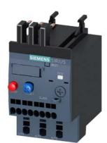
Overload relay 3.5...5.0 A Thermal For motor protection Size S00, Class 10 Contactor mounting Main circuit: Spring-type terminal Auxiliary circuit: spring-type terminal Manual-Automatic-Reset
