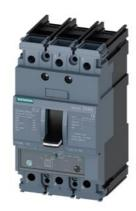
circuit breaker 3VA5 UL frame 125 breaking capacity class S 25kA @ 480 V 3-pole, line protection TM240, ATAM, In=60A overload protection Ir=48A ...60A short-circuit protection Ii=5...10 x In nut keeper kit on both sides
