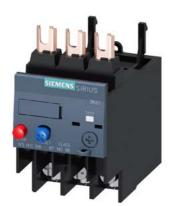
Overload relay 3.5...5.0 A Thermal For motor protection Size S0, Class 10 Contactor mounting Main circuit: Ring cable lug Auxiliary circuit: ring cable lug Manual-Automatic-Reset
