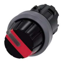
Selector switch, illuminable, 22 mm, round, plastic with metal front ring, red, Rotary knob, 2 switch positions O-I, latching, actuating angle 90°, 10:30h/13:30h, with laser labeling, upper case
