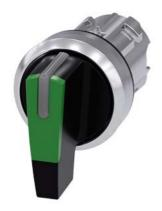
Selector switch, illuminable, 22 mm, round, metal, shiny, green, selector switch, long, 3 switch positions I>O<II, momentary contact type, actuating angle  $2x45^{\circ}$ , 10:30h/12h/13:30h, Z=50-unit packaging
