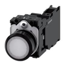
Illuminated pushbutton, 22 mm, round, plastic, white, pushbutton, flat, momentary contact type, with holder, 1 NO+1 NC, LED module with integrated LED 24 V AC/DC, spring-type terminal, with laser labeling, inscription or symbol Customer-specific selection with SIRIUS ACT configurator (CIN)
