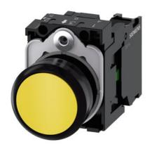
Pushbutton, 22 mm, round, plastic, yellow, pushbutton, flat, momentary contact type, with holder 1 NO, screw terminal, with laser labeling, upper case and lower case, always upper case at beginning of line
