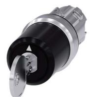
Key-operated switch BKS, 22 mm, round, metal, shiny, lock number S1, with 2 keys, 3 switch positions I>O<II, momentary contact type, actuating angle 2x45°, 10:30h/12h/13:30h, key removal O, Z=50-unit packaging
