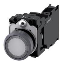
Illuminated pushbutton, 22 mm, round, plastic with metal front ring, clear, pushbutton, flat, momentary contact type, with holder, 1 NO+1 NC, LED module with integrated LED 24 V AC/DC, spring-type terminal, with laser labeling, upper case and lower case, Always upper case at the beginning of the word
