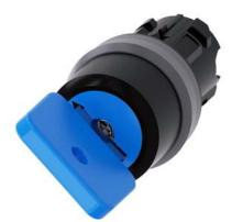
Key-operated switch O.M.R, 22 mm, round, plastic with metal front ring, lock number 73038, blue, with 2 keys, 2 switch positions O-I, latching, actuating angle 90°, 10:30h/13:30h, key removal O, with laser labeling, upper case
