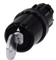
key-operated switch Siemens, 22 mm, round, plastic, special lock, with 2 keys, 3 switch positions I-O<II, left latching, momentary contact type on the right, actuating angle  $2x45^{\circ}$ , 10:30h/12h/13:30h, key removal O
