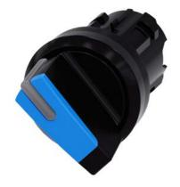
Selector switch, illuminable, 22 mm, round, plastic, blue, selector switch, short, 2 switch positions O-I, latching, actuating angle 90°, 10:30h/13:30h, with laser labeling, lower case
