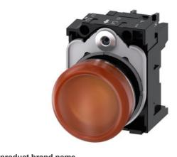
Indicator lights, 22 mm, round, metal, shiny, amber, lens, smooth, with holder, LED module with integrated LED 24 V AC/DC, screw terminal, with laser labeling, upper case and lower case, always upper case at the beginning of the word
