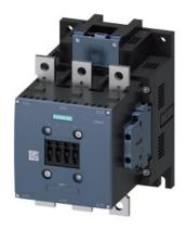
power contactor, AC-3 265 A, 132 kW / 400 V AC (50-60 Hz) / DC operation 21-27.3 V AC/DC auxiliary contacts 2 NO + 2 NC 3-pole, frame size S10 busbar connections drive: electronic with PLC interface 24 V DC screw terminal
