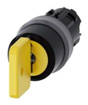
Key-operated switch O.M.R, 22 mm, round, plastic with metal front ring, lock number 73033, yellow, with 2 keys, 3 switch positions I-O-II, latching, actuating angle 2x45°, 10:30h/12h/13:30h, Key removal I+O+II, with laser labeling, upper case
