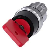
Key-operated switch O.M.R, 22 mm, round, metal, shiny, lock number 73037, red, with 2 keys, 2 switch positions O-I, latching, actuating angle  $90^{\circ}$ , 10:30h/13:30h, key removal O+I, Z=50-unit packaging
