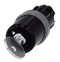
key-operated switch Siemens, 22 mm, round, plastic with metal front ring, lock number SSG10, with 2 keys, 2 switch positions O-I, latching, actuating angle 90°, 10:30h/13:30h, key removal O+I, with laser labeling, upper case
