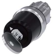
Key-operated switch BKS, 22 mm, round, metal, shiny, Lock No. E9 (VW), without key, 2 switch positions O-I, latching, actuating angle 90°, 10:30h/13:30h, key removal O, with laser labeling, upper case and lower case, always upper case at beginning of line
