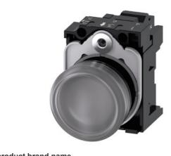
Indicator lights, 22 mm, round, plastic, clear, lens, smooth, with holder, LED module, with integrated LED 230 V AC, spring-type terminal, with laser labeling, inscription or symbol Customer-specific selection with SIRIUS ACT configurator (CIN)
