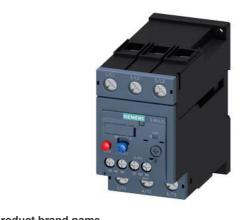
Overload relay 36...45 A Thermal For motor protection Size S2, Class 10 Stand-alone installation Main circuit: Screw Auxiliary circuit: Screw Manual-Automatic-Reset
